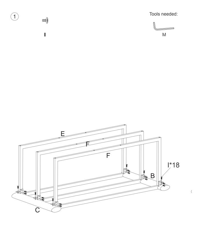
1. Attach frames (E&F) to the pillars (B&C) with screws (I).
